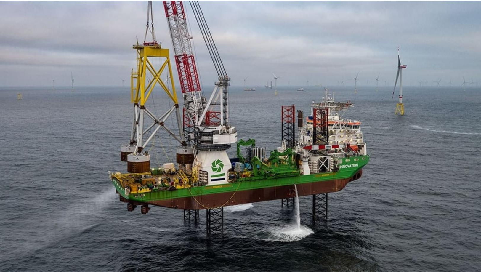
Suction Bucket Jacket on GeoSeas heavy lift vessel Innovation to be lifted and placed on the seabed at Borkum Riffgrund 2 and thereafter penetrated into place by suction inside the three foundation buckets.
