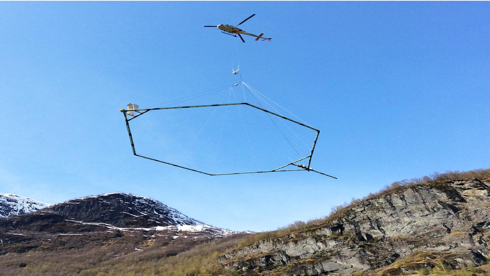
The antenna which registers the ground conditions hangs below the helicopter running along the area to be investigated
