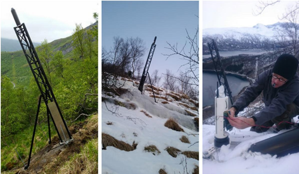
*The radio tower which is located close to the respective avalanche paths are bolted to the rock roughly perpendicular to the hillside inclination. NGI's Yme Kvistedal (right picture) captured while connecting wires from the geophones which registers vibrations from Avalanches.*
